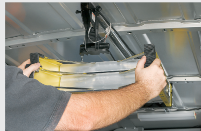
3 Raise the foot of the ladder to secure it to the catch bracket.
