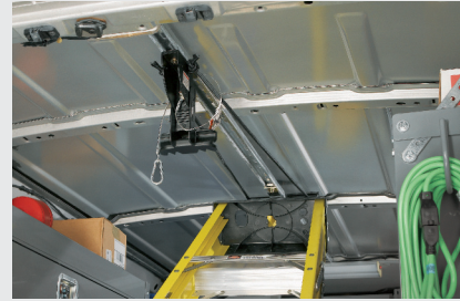
1 Hook the ladder onto the receiving pin.
