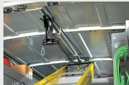
2 Slide the ladder forward along the rail.
